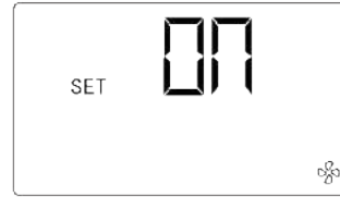
Fig.4.5-6 Ventilation function is on
